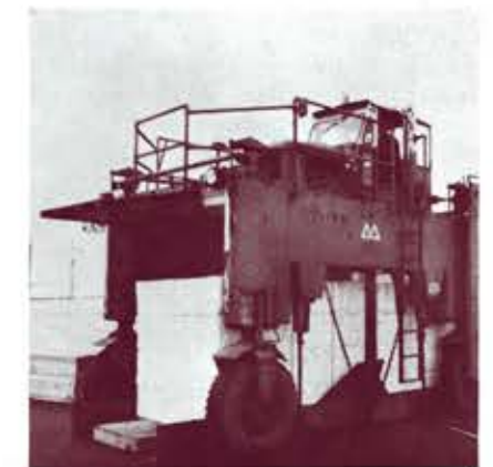
The big straddle carriers aren't geared to carry a full load uphill, as they have to get from the pulp room to the outside storage area, but they still manage to haul 30-odd tons a trip. The carrier shown above is being operated by Driver Wally McCallum.
