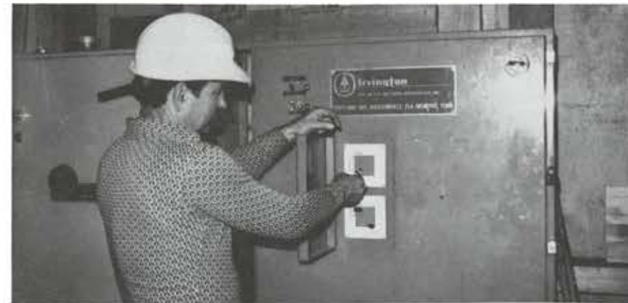
Planer Foreman Johnny Sevcov, setting the controls of the sorting and grading programmer to turn out the scheduled length and grade of lumber.
