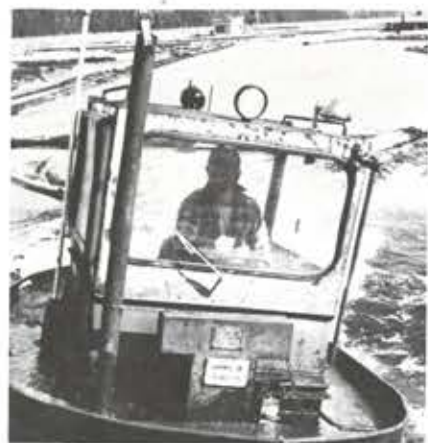
Scotty Thompson in his stubby 'boom buggy' [a workhorse dozer boat]. Highly maneuverable, the dozers not only push logs but can ride right over them. Naturally the prop is completely caged to protect it from such rough riding.
